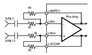
Figure 10. External Connection Example (differential input)
