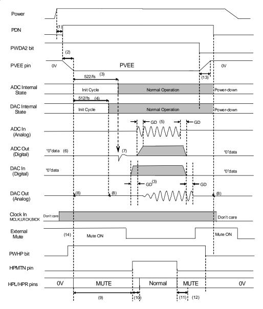
Figure 17. Power-up/down Sequence Example
