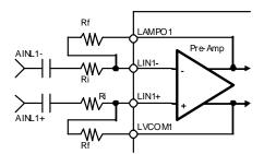
Figure 1. ADC Input Circuit
