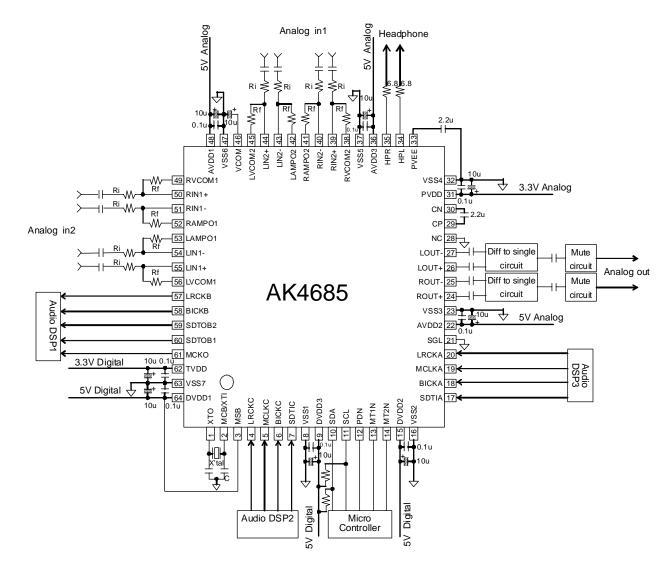
Figure 28. Typical Connection Diagram (Master Mode)
