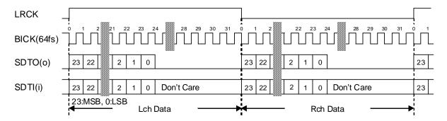
Figure 7. Audio Data Timing (SDTO: Mode0/2, SDTI: Mode2)
