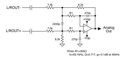
Figure 13. External 2<sup>nd</sup> order LPF Circuit Example (using op-amp with dual power supplies)
