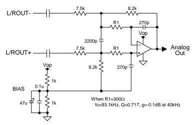
Figure 12. External 2<sup>nd</sup> order LPF Circuit Example (using op-amp with single power supply)
