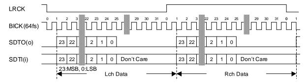
Figure 8. Audio Data Timing (SDTO: Mode1/3, SDTI: Mode3)
