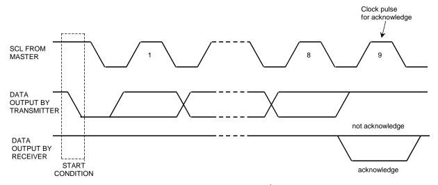
Figure 21. Acknowledge on the I<sup>2</sup>C-bus
