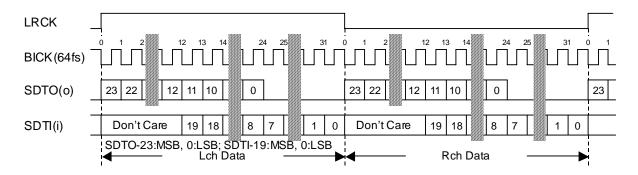
Figure 5. Audio Data Timing (SDTO: Mode0/2, SDTI: Mode0)
