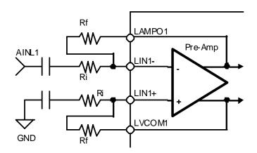
Figure 11. External Connection Example (single-ended input)
