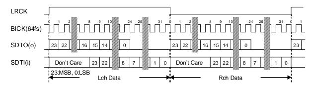
Figure 6. Audio Data Timing (SDTO: Mode0/2, SDTI: Mode1)
